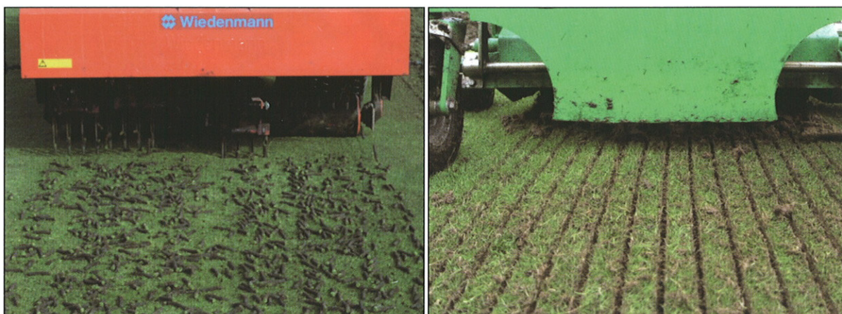
Hollow coring (left) and scarification (right) are the main mechanical operations to remove thatch accumulations
